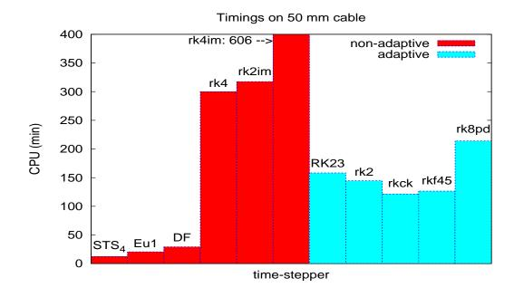
Figure 3: Timings of all eleven schemes on 50mm cable. Non-adaptive (red) and adaptive (cyan) schemes.
