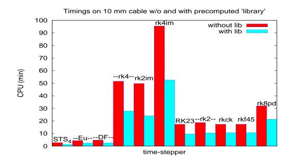
Figure 2: Timings of all eleven schemes on 10mm cable, without (red) and with precomputed library (cyan). Precomputing achieves almost 100% speedup on most schemes.
