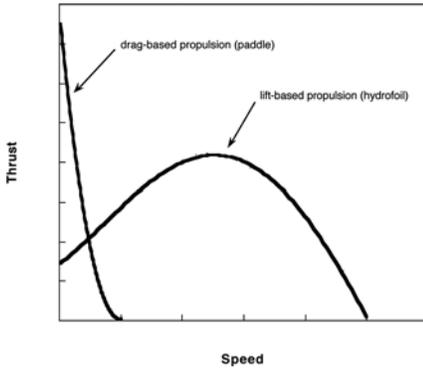
systems is limited by swimming speed (Figure 1). Drag-based paddling operates most effectively at low speeds, whereas lift-based hydrofoils perform best at higher speeds. As a flow field needs to be established for a lifting surface to work, hydrofoils are limited in use to conditions where the body of an animal is already in motion. Paddles can be used when the body is stationary. A paddle of large area can impart sufficient momentum to
