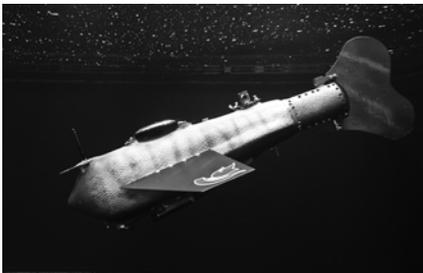
A substantial increase in efficiency in animals can be realized by using passive gliding. Negatively buoyant fish conserve energy by gliding downward with no propulsive motions and then regaining altitude by actively swimming. This strategy is used by AUV gliders (Figure 5; Tan, 2011).
